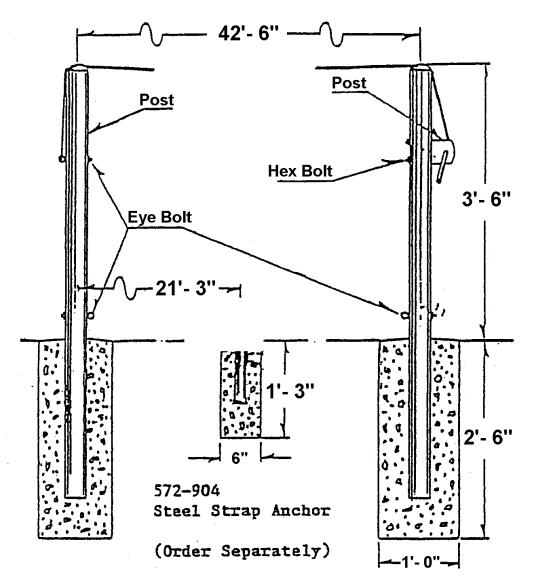
SPECIFICATIONS: Posts are  $3.5\ \text{OD}\ x\ 8$  Gage galvanized steel tubing with a cast aluminum cap and ratchet type net reel.
